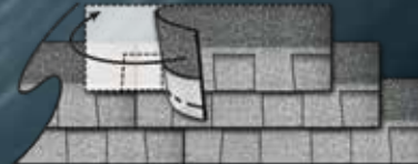
SEALANT STRIPS ARE LOCATED ON THE FRONT OF MANOIR SHINGLES.
