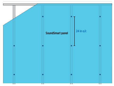
• Using 32 mm (1 ¼ in) Type-S screws, fasten the SoundSmart panel into studs @ 24" o/c.
